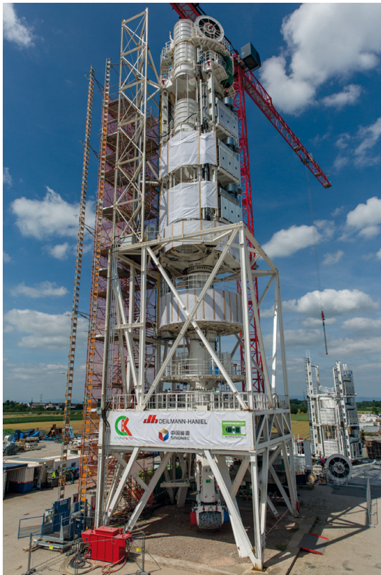
Fig. 2: Shaft Boring Road Header (SBR) by Herrenknecht AG Source: Herrenknecht AG
