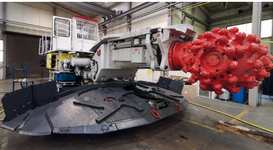
Fig. 4: Boom-type roadheader refurbished by CST
