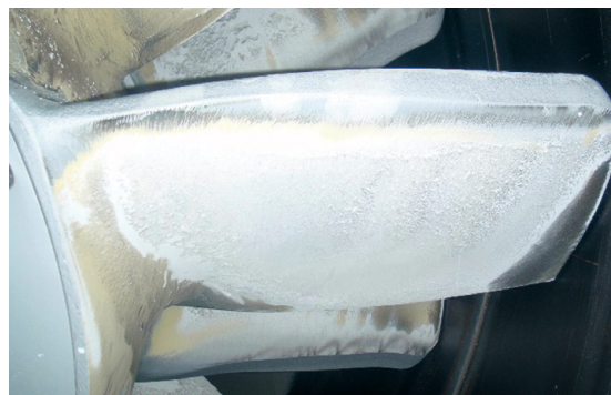
Fig. 10: Wear due to dust
