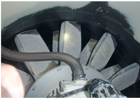
Fig. 9: Impeller conveying dust
