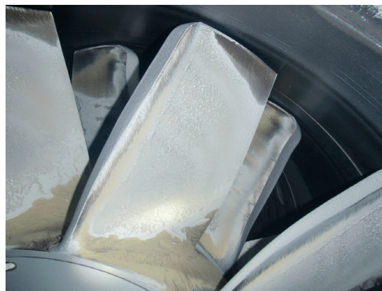
Fig. 11: Severe abrasion at the blade tips
