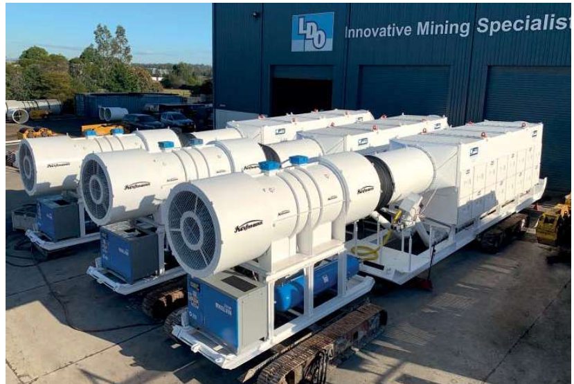
The axial fans produced by Korfmann Lufttechnik have impellers measuring 300 to more than 3,700 mm in diameter. (Photo: CFH Group)
